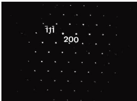
Figure 22 Characteristic dot pattern diffraction image produced by a single crystal
