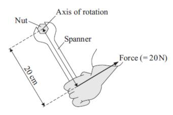
Calculate the spanner's turning effect in newton metres.
