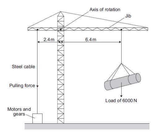
The purpose of the motors and gears is to change the pulling force in the steel cable. This is done so that the jib stays horizontal whatever the size of the load or the position of the load.
