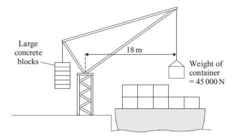
(a) Use the equation in the box to calculate the moment of the container which is being loaded.
