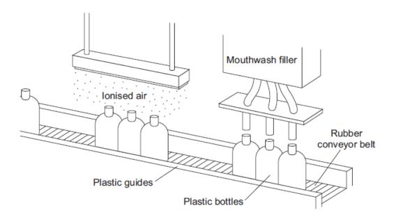
The company came up with a solution to the problem. Before the bottles reach the filler, they pass through a stream of ionised air. The ions in the air neutralise the charge on the bottles.
