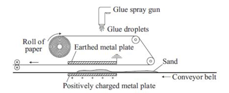
Glue is sprayed onto a moving strip of paper. As the glue leaves the spray gun, the glue breaks up into tiny negatively charged droplets which coat the paper. The sticky paper passes between two metal plates. Sand moving on a conveyor belt also passes between the metal plates.
