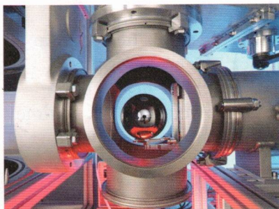
▲ Figure 1: An Avogadro Project sphere [in the centre of this measuring machine] is made of pure silicon and is the most spherical object ever made by humans – it is so perfectly spherical that if it were scaled up to the size of Earth, with a radius of 6370 km, its highest point would only be around 2 m above its lowest point
