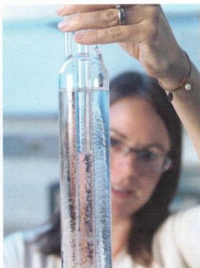
▲ Figure 1 The three phases of water – solid, liquid, and gas – are in thermal equilibrium inside this triple-point cell: the ice does not melt, the water vapour does not condense
