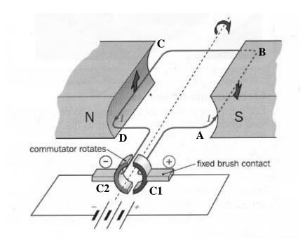
The split-ring commutator swaps the contacts with the brushes every half turn. This changes the direction of current in the coil every half turn and enables the coil to keep on rotating in the same direction.
