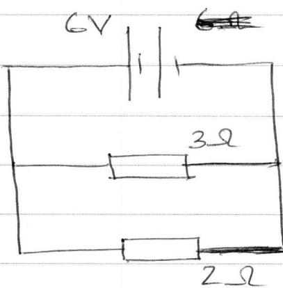
Work out the current flowing through the 3Ω resistor.
