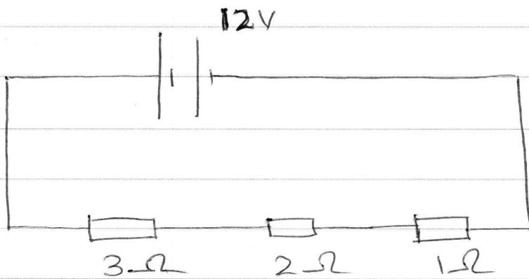
Work out the current flowing through the 3Ω resistor.
