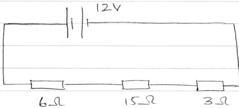
Calculate the voltage across the 15Ω resistor.
